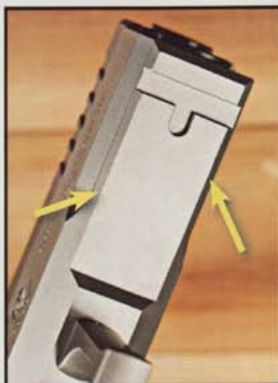
Note an universal accessory rail for lights, lasers.
