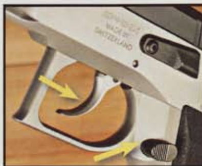
Smooth-faced trigger works well in DA mode, mag button is extended for a positive mag dump.
